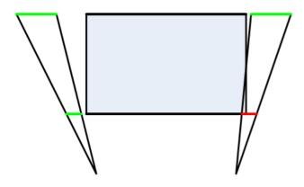
Figure 3: Two of the possible results of packet-box separation. Green - frustrum misses; Red - frustum intersects.
