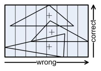
Figure 2: Object vs. centroid AABB
